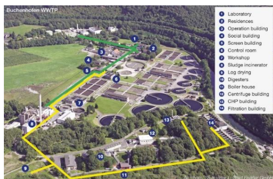
Figure 8-10: Heat grid at Buchenhofen
